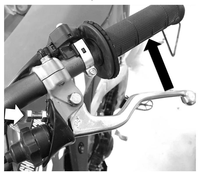
• Backing your adjuster bolt farther out will push the lever farther from the bar and allow for a further reach point.
